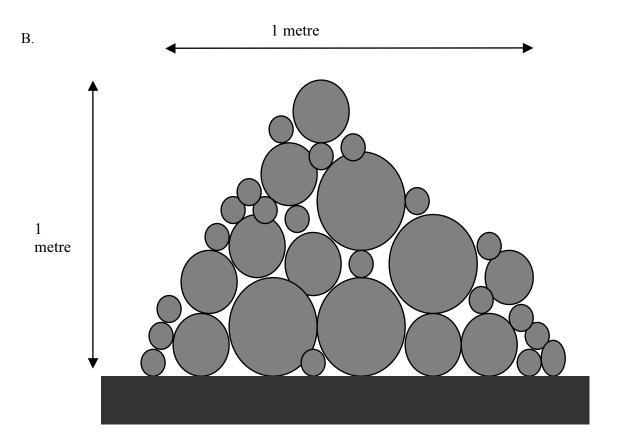
**Figure 28.** Generalised design of the rock-line artificial habitats installed at Lake Navarino.
