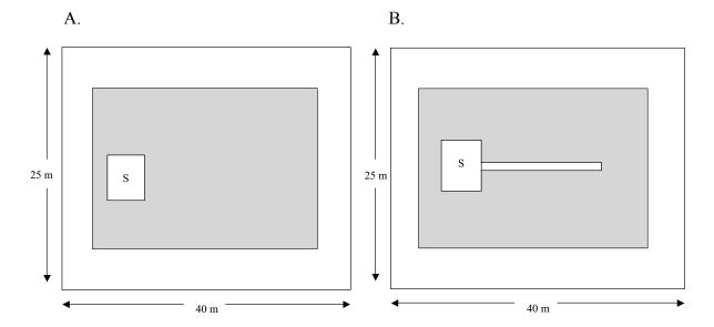
**Figure 17.** Schematic design of; A.) a typical 1,000 m² marron grow-out pond with 3 x 3 m concrete sump (S); B.) a 1,000 m² large nursery pond constructed at the Pemberton Freshwater Research Centre to support the current project, with a 3 x 3 m concrete sump (S) and a 9.6 m concrete channel to allow the aggregation of large numbers of juvenile marron. From Molony (2002c).
