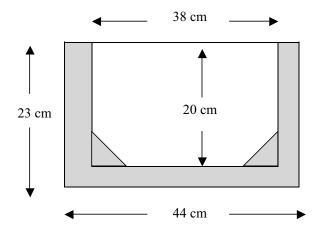
**Figure 18.** Details of the cross-section of the 9.6 m concrete drain available as 'small spoon drain section' from many concrete product manufacturers in 1.2 m lengths. From Molony (2002c).
